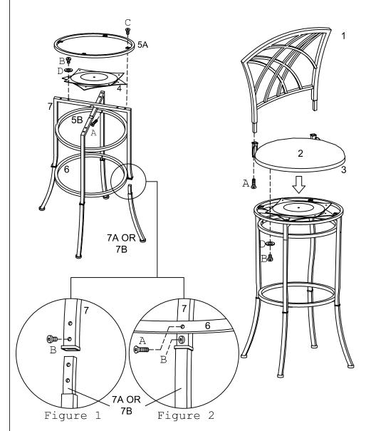
Step 1. Attach both Leg Assemblies 7 by crossing them between each other and attach Inner Ring 5B to inside of each leg by using (4) Allen Bolt A. Only hand tighten bolts for this step.
